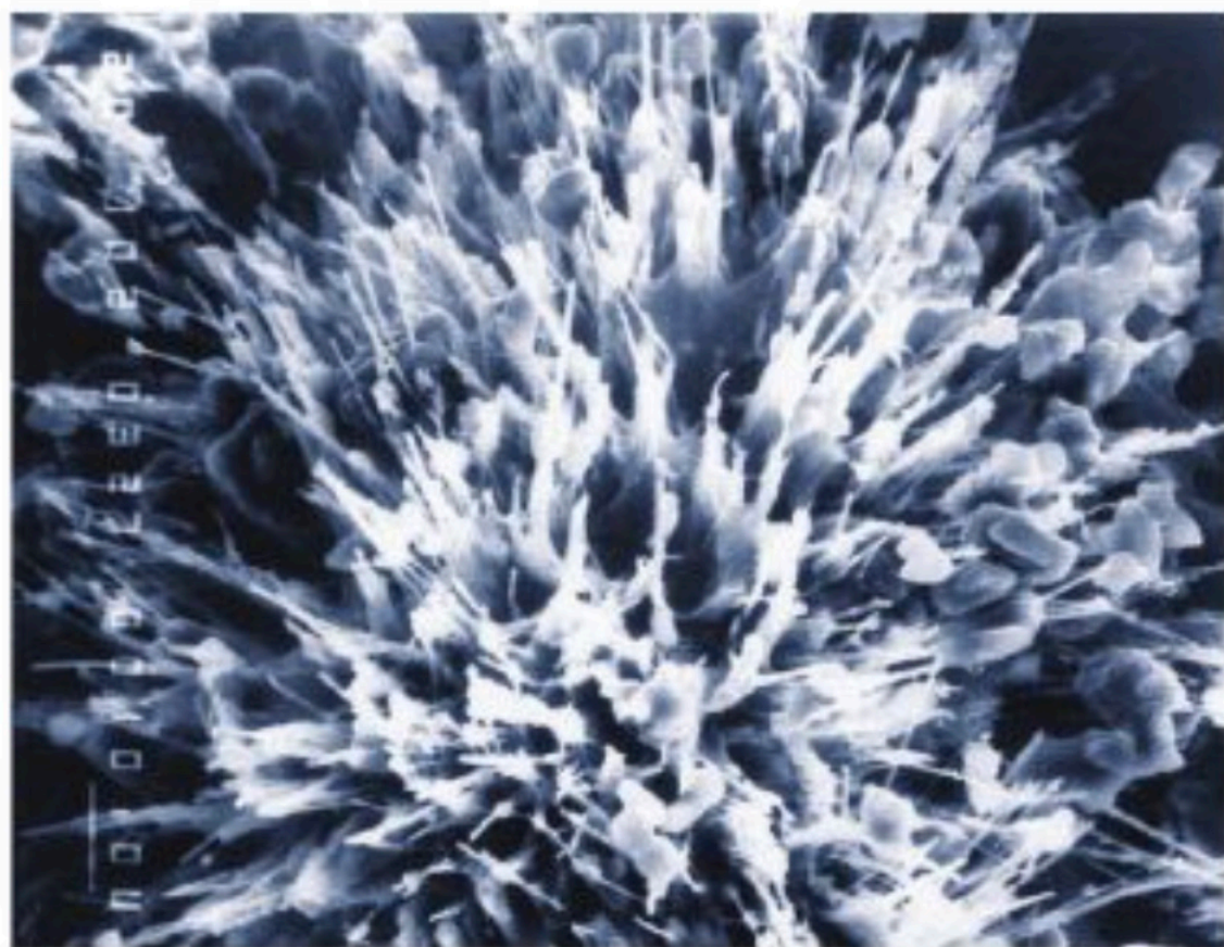
SEM view of a concrete pore as it fills with multiplicative crystalline formation.
