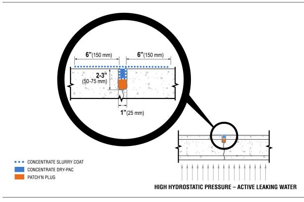
**STEP 1:** Chip out crack/joint in a "U" shaped slot as per the drawing shown above. The slot is to be 1" (25 mm) wide and 2" - 3" (50 - 75 mm) deep. A "V" shaped slot is not acceptable. The slot may be saw cut instead of chipped but ensure that the slot is dovetailed or otherwise shaped such that there will be mechanical interlock of materials placed into the slot at a later stage.
