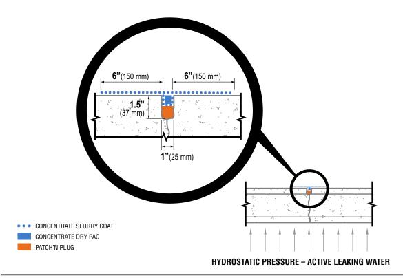
**STEP 1:** Chip out crack/joint in a "U" shaped slot as per the drawing shown above. The slot is to be 1" (25 mm) wide and at least 1.5" (37 mm) deep. A "V" shaped slot is not acceptable. The slot may be saw cut instead of chipped but ensure that the slot is dovetailed or otherwise shaped such that there will be mechanical interlock of materials placed into the slot at a later stage. Areas with the most water flow should be identified and chipped slightly deeper.
