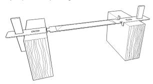
Most flat bar snap ties are designed to break back approximately 1/4" (6 mm) below the surface of the concrete.
