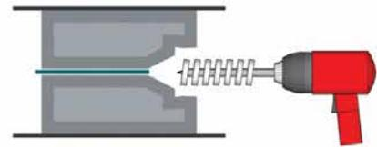
**STEP 2:** Remove all loose material within the void. Thoroughly clean and saturate this area with water. Allow water to soak into concrete and then remove all surface water. All surfaces should be left saturated-surface-dry (SSD – wet but with no glistening water).
