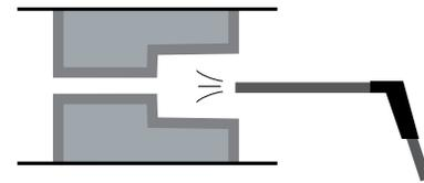
**STEP 3:** Compact a blend of 3 parts Xypex Concentrate and 1 part Xypex Patch'n Plug made to a mortar consistency into the bottom of the prepared section of the hole to form a plug. The plug is to be 2" - 3" (50 - 75 mm) thick. There must remain at least a 8" (200 mm) of space between the top of the plug and the surface of the concrete element. Remove any of the plugging material from the outer surface of the concrete wall or element by scrubbing or grinding.
