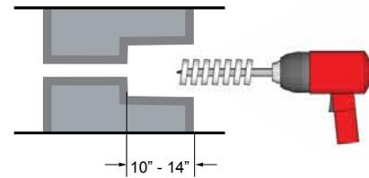
**STEP 2:** Remove all loose material within the void. Thoroughly clean and saturate the void with water. Allow water to soak into concrete and then remove all surface water. All surfaces should be left saturated-surface-dry (SSD – wet but with no glistening water).
