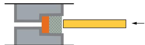
**STEP 5:** Cure by keeping moist for two to three days. Open to water contact as per Xypex guidelines.
