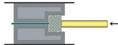
**STEP 4:** Cure by keeping moist for two to three days. Open to water contact as per Xypex guidelines.
