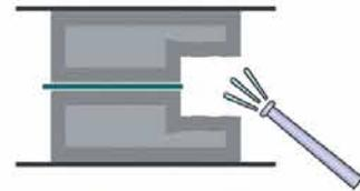
**STEP 3:** Fill the void to the surface with Xypex Megamix II with Bio-San mixed to a stiff mortar consistence. Use an appropriate method to get full compaction of the Xypex Megamix II with Bio-San.
