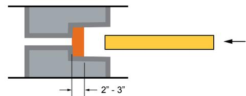
**STEP 4:** Fill the remaining void to the surface with Xypex Megamix II with Bio-San mixed to a stiff mortar consistence. Use an appropriate method to get full compaction of the Xypex Megamix II with Bio-San.
