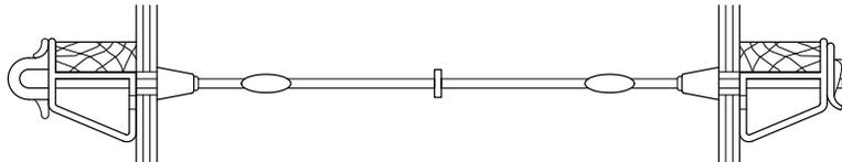
**STEP 1:** Using a hammer drill, or chisel bit that is slightly larger than the outside diameter of the cone, drill out or chip out the cone shape to the full depth of the indentation leaving a rough surfaced, straight-sided void.
