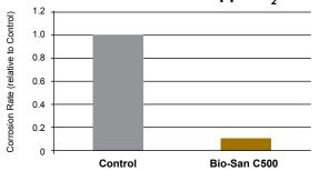
Corrosion Rate at 50 ppm H<sub>2</sub>S
