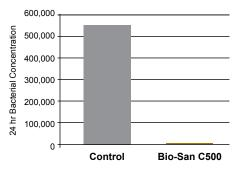
Concrete was cast in 100 x 200 mm cylinders with both control and treated mixes. A wastewater facility was chosen that had elevated  $H_2S$  levels and substantial existing MIC corrosion damage.Test samples were suspended in the air space of the tank for 10 years. Exposure trials showed that treated concrete had nine times less concrete mass loss compared to control samples.
