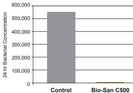
Concrete was cast in 100 x 200 mm cylinders with both control and treated mixes. A wastewater facility was chosen that had elevated H<sub>2</sub>S levels and substantial existing MIC corrosion damage. Test samples were suspended in the air space of the tank for 10 years. Exposure trials showed that treated concrete had nine times less concrete mass loss compared to control samples.
