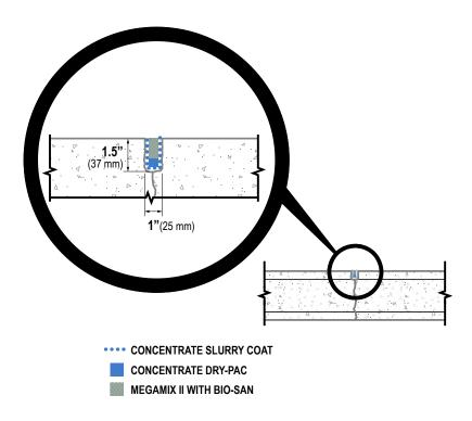
For repairs of cracks on the dry or negative side, including actively leaking cracks, use Xypex's standard crack repair procedures. Crack repairs made on the dry or negative side will not adversely impact the anti-microbial nature of the Xypex Bio-San C500 concrete element.
