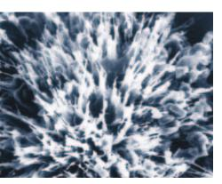
In crystalline PRAHs, the reactive chemicals use water to migrate into and travel down the capillaries of the concrete. The process initiates a chemical reaction involving the crystalline chemicals, moisture, and the by-products of cement hydration, which forms a new non-soluble crystalline structure. This integral structure fills the capillary tracts and renders the concrete waterproof.
