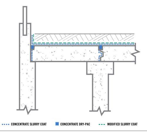
**STEP 1:** Clean joint thoroughly. Apply Xypex Concentrate slurry to joint surface at the rate of 2.0 lb./sq.yd. (1.0 kg/m²).
