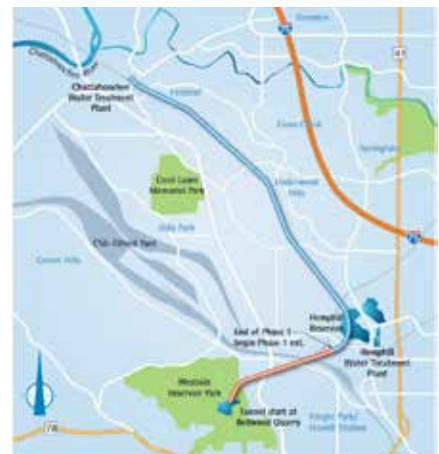
Fig 3 – The $368 million Atlanta Water Program has included a five-mile TBM tunnel from the Bellwood Quarry to the Chattahoochee River, connecting the quarry to the Hemphill and Chattahoochee water treatment plants. The project has increased the city’s raw water reserve from three days to more than 30 days.
