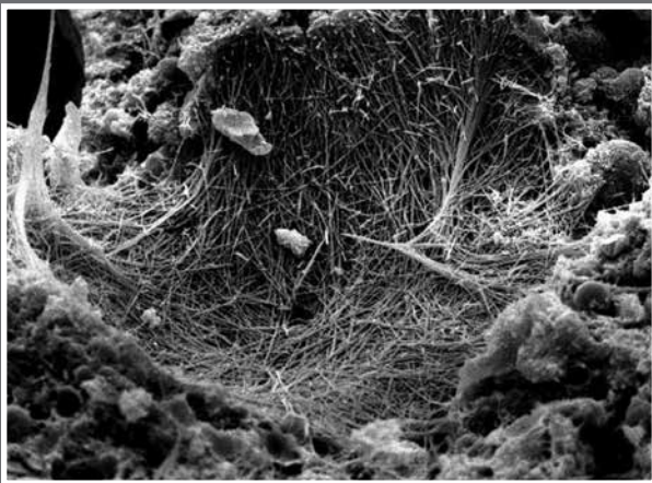
XYPEX TREATED CONCRETE
