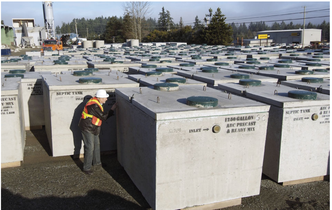
Currently a significant portion of sewage in North America is treated with septic tanks
