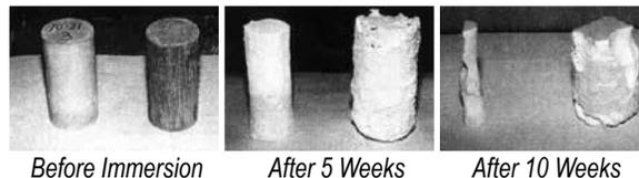
Xypex-treated mortar and untreated mortar were measured for acid resistance after exposure to a 5% H<sub>2</sub>SO<sub>4</sub> solution for 100 days. Xypex suppressed concrete erosion to 1/8 of the reference samples.
